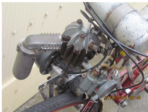
Trojan Mini Motor installation, very well engineered by Neil including a Soles Roller.
